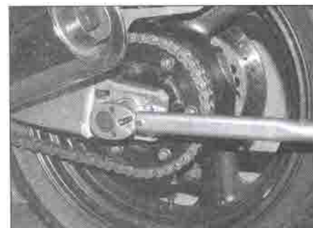
1.14 Tighten the axle nut to the specified torque
