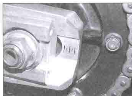
1.12c ... or back edge of the adjustment marker with the marks on the swingarm. On this bike you would use the front edge as the rear edge has not yet reached the alignment marks
