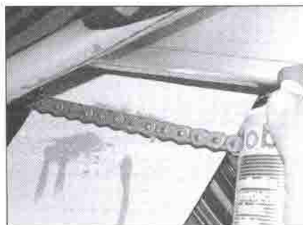
1.16 Apply the lubricant to the overlap between the sideplates. Note the use of a piece of card to prevent lubricant contacting the tyre
