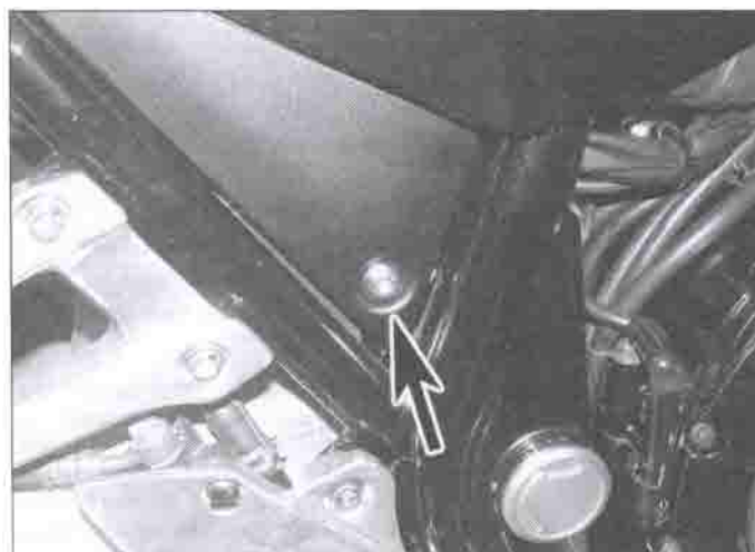
3.3a Unscrew the bolt (arrowed) ...
