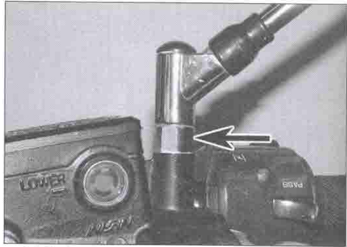
6.1 Slacken the locknut (arrowed) then unscrew the mirror
