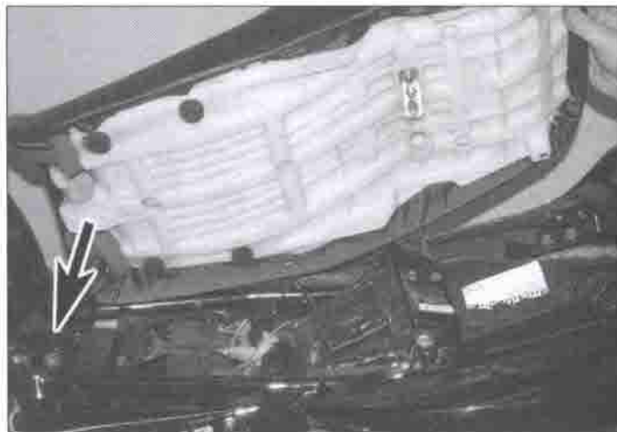
2.2 The tab locates under the tank bracket
