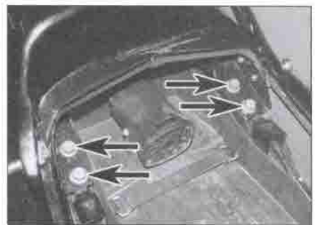
4.2c Slacken the bolts (arrowed) if the grab-rail is tight
